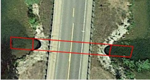
To maximize the air gap through the culvert, the grade on Hwy 64 needs to be raised 2-3 feet. This grade rise will need to occur over a mile-long section of highway. While construction work is going on, traffic will be detoured around Cty 25.
